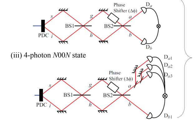
Intensity  $\sim \sin N \Delta \phi$ Sensitivity  $\sim \frac{1}{N}$
