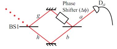
Given N photons, how precisely can the optical phase be measured?
