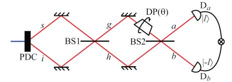
$$|\psi_{2}^{l}\rangle = \sqrt{\frac{1}{2}} \left[ |1\rangle_{s_{+l}} |1\rangle_{i_{-l}} + |1\rangle_{s_{-l}} |1\rangle_{i_{+l}} \right] = \sqrt{\frac{1}{2}} \left[ \hat{s}_{+l}^{\dagger} \hat{i}_{-l}^{\dagger} + \hat{s}_{-l}^{\dagger} \hat{i}_{+l}^{\dagger} \right] |\text{vac}\rangle$$
